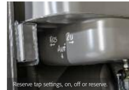
The fuel reserve tap is in the engine room.
